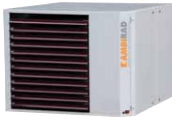
The UESA range of room sealed fully condensing unit heaters utilises patented MacroChannel heat exchanger technology to deliver up to 104% thermal efficiency (based on net CV).
